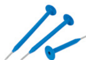
Insulation dowel SFS RP50/BS-4,8 wood (XFM 006) – distancer/fastener. The same product works as a fastener for the insulation and as a distancer for 180 mm thick wind-resistant insulation.
