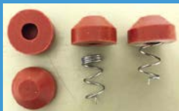
Option 2: Single spacers with springs recommended for pipes with ≤30 mm diameter and smaller areas of insulation (e. g. inspection hatches) as well as pipe elbows
