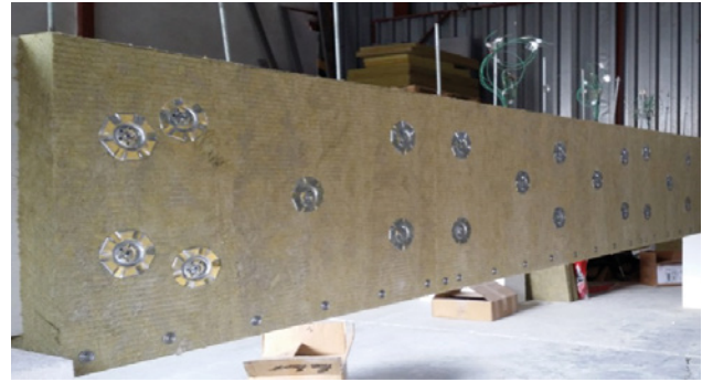
Fire protected concrete beam.
