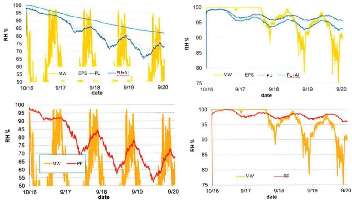
**Figure 6. Simulation results on the relative humidity levels on the interior boundary (left) and on the exterior boundary (right) of the thermal insulation in a concrete sandwich wall. Observe that the stone wool curves in the top and bottom graphs are the same to guide the eye of the reader. The figures are sourced from the VTT studies [5] [6].**
