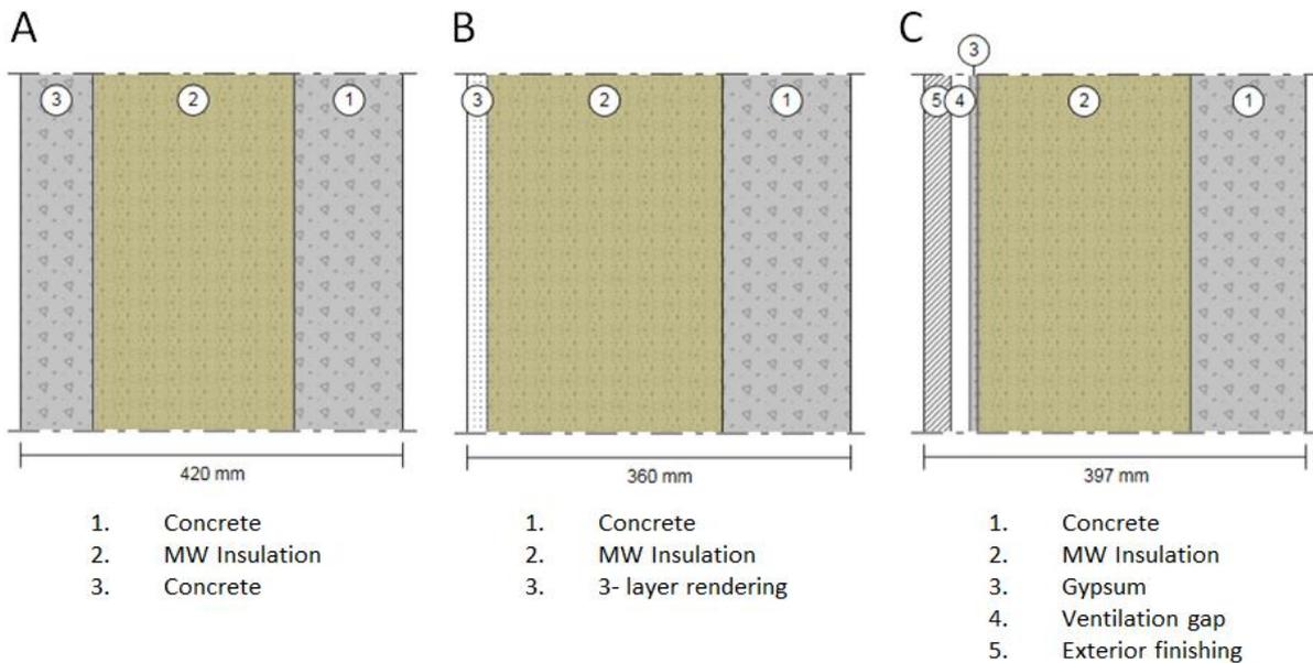
**Figure 1. The intersections of the wall structures used in simulations: A) a concrete sandwich panel, B) a rendered façade, and C) a ventilated façade. Constructions based on data given by Ojanen [5] [6].**
