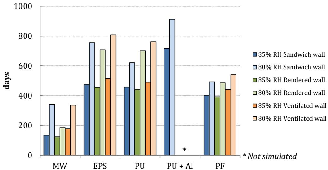
**Figure 4.** Time needed for the interior concrete layer (thickness = 120 mm) to reach the average moisture contents corresponding to 85 % RH or 80 % RH for the three studied wall structures given in Figure 1. The data is collected from [5] [6].
