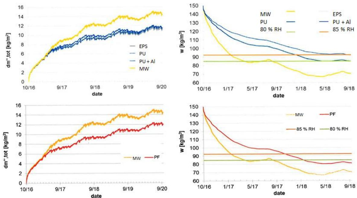
**Figure 3. Total mass of moisture dried out from the structure (left) and the average moisture content levels of the inner concrete slabs (right) for a concrete sandwich wall with different insulation materials. The horizontal lines represent 80 % RH and 85 % RH humidity levels. Observe that the stone wool curves in the top and bottom graphs are the same to guide the eye of the reader. The figures are sourced from the VTT studies [5] [6].**
