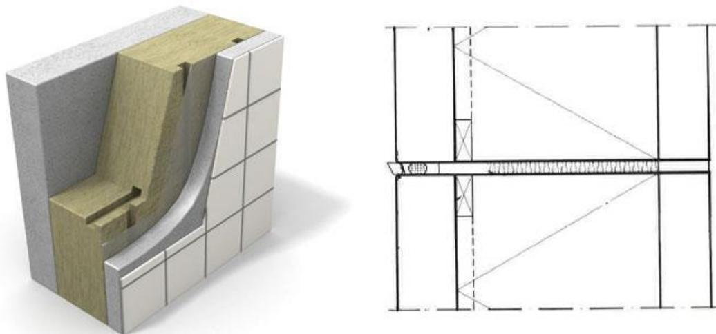
**Figure 2. Ventilated stone wool insulation system used in concrete sandwich panel: a 3D illustration of the grooved insulation on the left and on the right a detail (side view section) from the air inlet/outlet pipes between the elements.**
