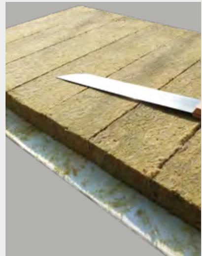
Mount the PAROC® Pro Lamella Mat Clad on the duct sides and back. In order to make the installation easier, a spray adhesive could be used. For the permanent mechanical fixation on the duct we recommend using welding pins; with a maximum distance of 300 mm. To ensure a uniform positioning of welding pins, we recommend using a corresponding template.
