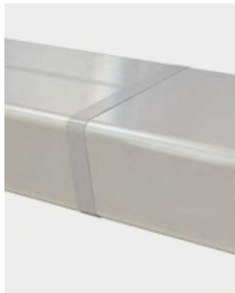
Always make sure that tape is applied without wrinkles and openings. Use a spatula to smoothen out any air bubbles. There must be no gaps or "pockets" where water can accumulate.
