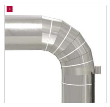
In order to effect a durable mechanical fixation of the pipe casing as prescribed by DN100, use additional SIGNODE strips or an alternative weatherproof plastic strip.
