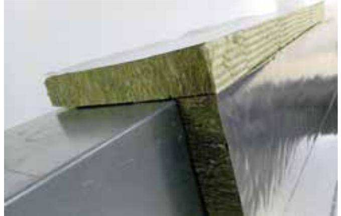
In order to follow requirements coming from DIN4140 standard related to a need of keeping min. 3% of gradient to protect a top surface of a rectangular ventilation duct against accumulation rainwater please put PAROC Pro Wedge (WR) and next on it install PAROC Pro Lamella (WR) Clad.
