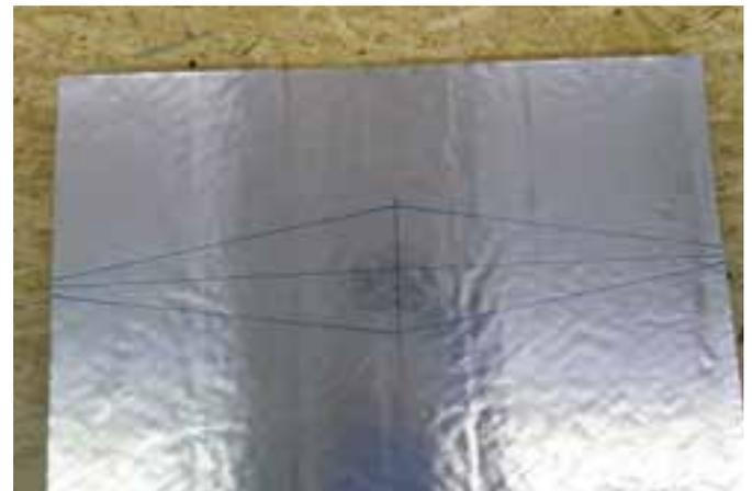
On both edges of the circumference, on the auxiliary line on both sides, mark half of the dimension "a";
