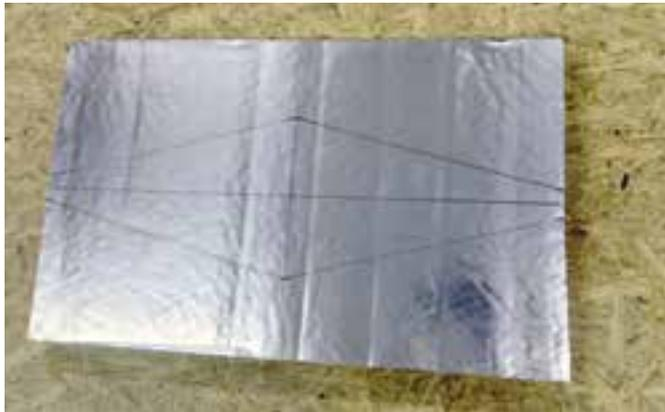
On both edges of the perimeter, on the auxiliary line, mark about 1/5 of the length of the elbow measured at the throat, diagonally, e.g. if the length is 210 mm, the dimension to be applied on both sides should be about 40 mm;
