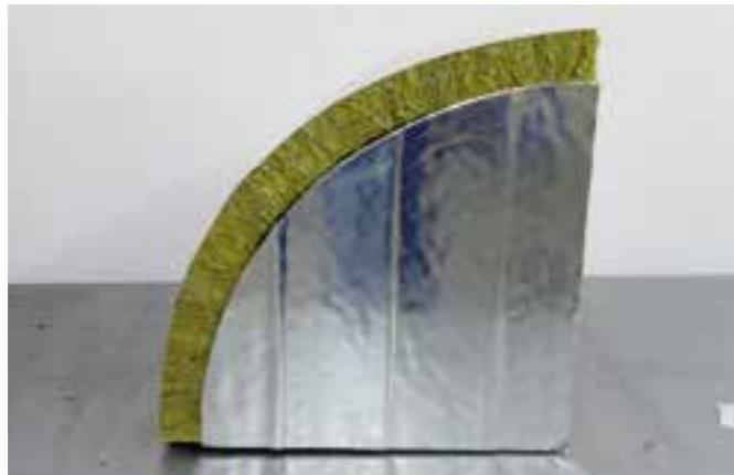
Add the value corresponding to two times the insulation thickness to the mat strip for the arc duct surface so you will not have to tape up the fold on the duct edge on the entire insulation thickness;
