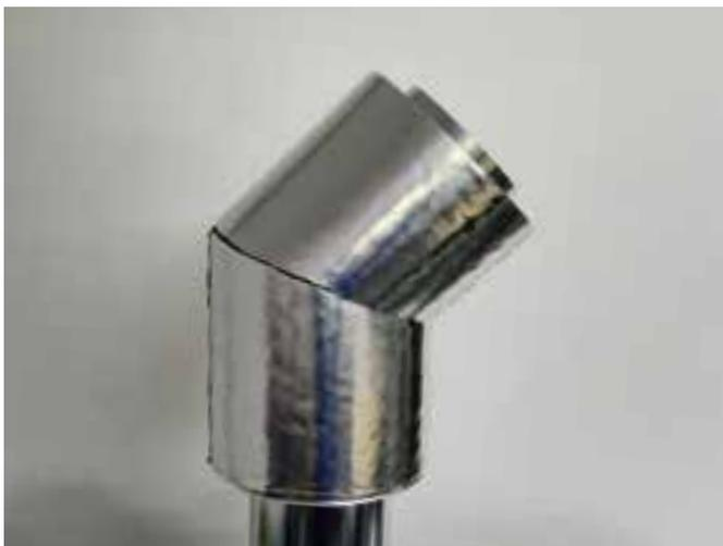
The cut out elements should be placed on the bend - the elbows below 90° - and the longitudinal and circumferential joints should then be covered with PAROC Clad Tape with the sealing compound.
