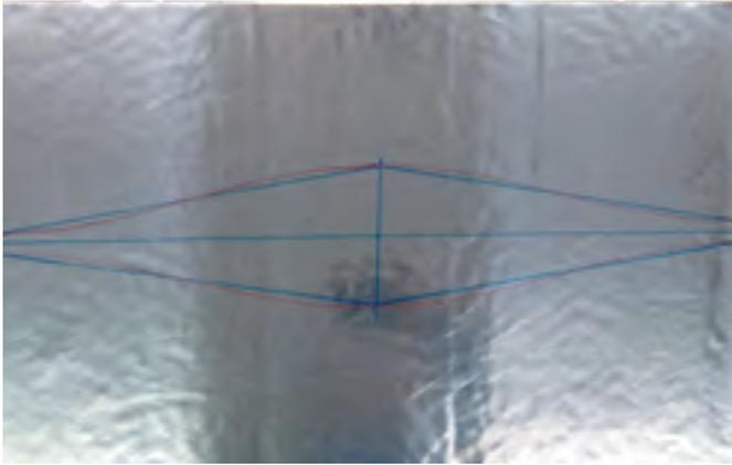
**6.** Cut out the resulting figure by duplicating, it depending on the number of segments in the elbow. To prevent waste, you can use the element cut out from the wool as a template by moving it half-way around the circumference. Then the folding will be alternately - once in the throat of the elbow, then on the outside of the elbow;
