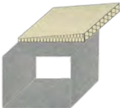
**STEP 2:** Installation of PAROC® Pro Lamella Mat Clad (on top of the Wedge)
