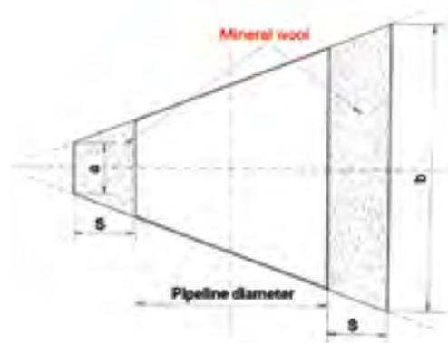
3. In the selected location, mark an auxiliary line (the symmetry of the middle element of elbow insulation); On the auxiliary line, mark the point corresponding to the half the length (circumference) of the mat; At the point on both sides, mark half of the dimension "b".
