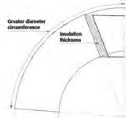
**3.** Cut out the mat element at a slanting angle so that after cutting out it may complete the insulation at the reduction spot;
