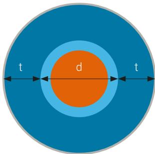
For round ducts with diameter below 1000 mm, the use of alternative solutions such as pipe sections or a lamella mat double-layer system is recommended. These alternatives offer greater material flexibility and may be more suitable for applications requiring bending, alignment, or adaptation during installation.
