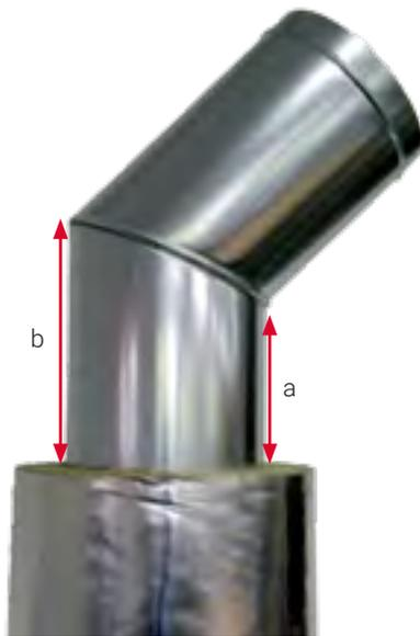
2. On both sides of the mat, draw arcs (with the radius corresponding to half the circumference of the insulated pipeline) that are tangential to the lowest spot "a" of the arc;
