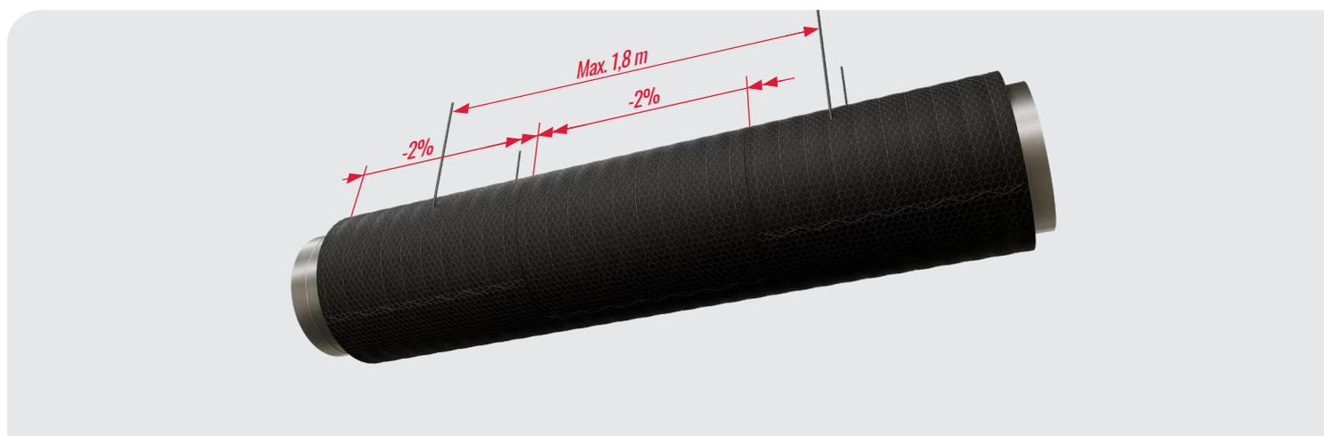
6. Place the remaining mats on the duct. The longitudinal joints of the adjacent mats are to be offset by a minimum of 100 mm. The last mat must be compressed against the wall with the fire sealant following the principles of 4.
