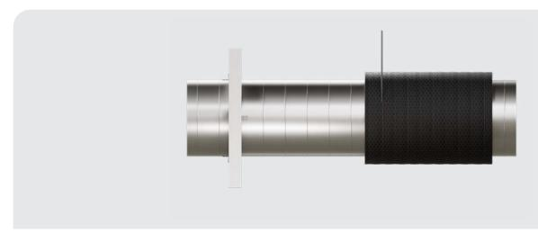
Install and stabilize the first mat adjacent to the wall. Unless the fire sealant is still wet, the wall surface must be primed with clean water and another layer of fire sealant applied to create a gluing layer for the insulation. Spread the fire sealant with a wet brush or spatula to make a soft layer approximately 1 mm thick. Immediately after, while the fire sealant is still wet, glue the insulation to the wall.
