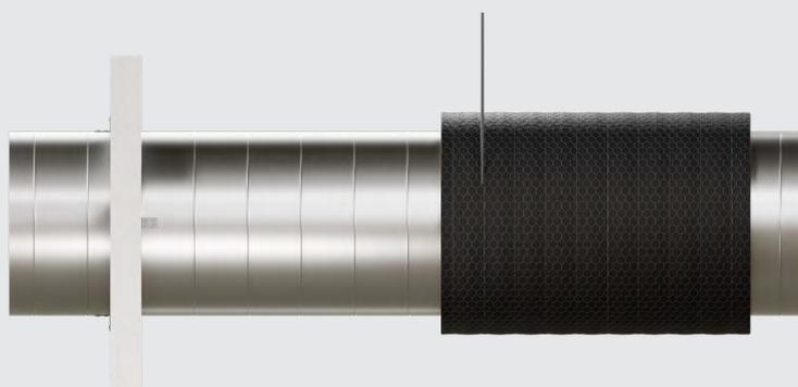
4. Install and stabilize the first mat adjacent to the wall. Unless the fire sealant is still wet, the wall surface must be primed with clean water and another layer of fire sealant applied where the edge of the insulation is in contact with the wall. Spread the fire sealant with a wet brush or spatula to make a soft layer approximately 1 mm thick. Immediately after, while the fire sealant is still wet, compress the insulation against the wall.
