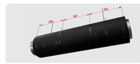
**9.** Install the wire loops around the insulated duct to secure its position, twisting the ends of each wire together. The spacing of the loops is a maximum of 150 mm; 50–100 mm from the wall.
