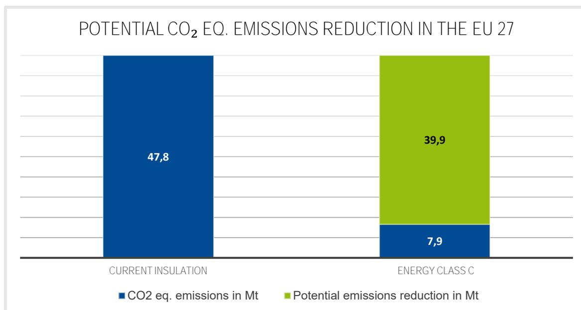
Figure 15: Comparing the potential CO<sub>2</sub> eq. emissions reduction in EU 27 – the situation today vs. the VDI 4610 energy class C scenario
