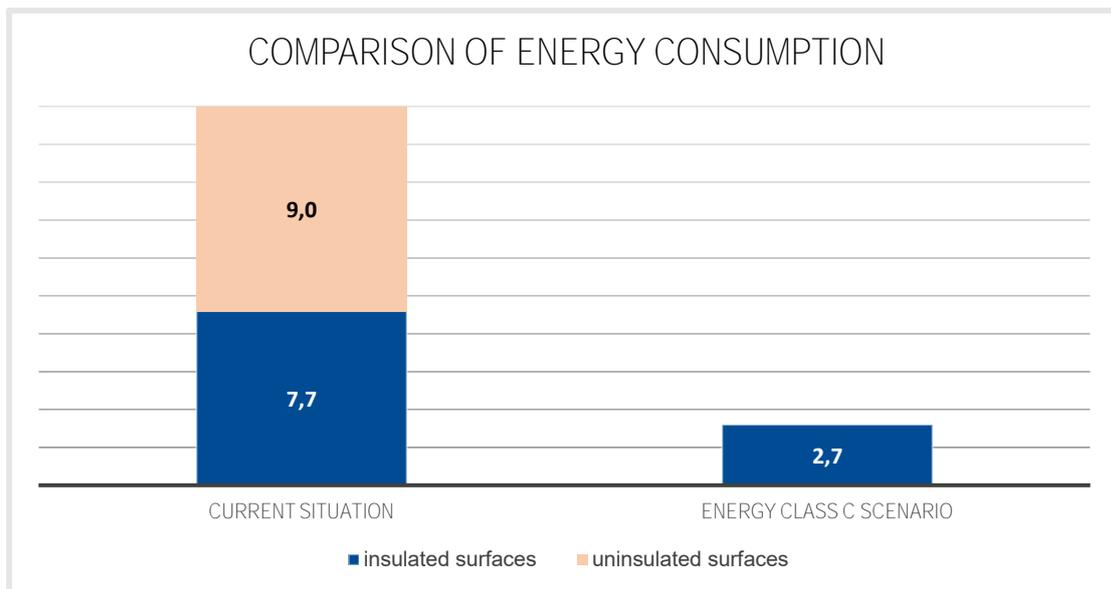
Figure 2: Energy savings if insulation systems are upgraded to VDI 4610 energy class C
