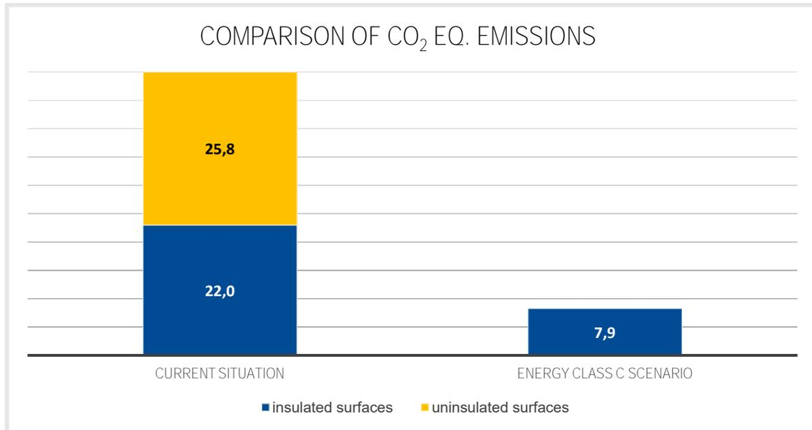
Figure 3: CO<sub>2</sub> eq. emissions reduction if insulation systems are upgraded to VDI 4610 energy class C
