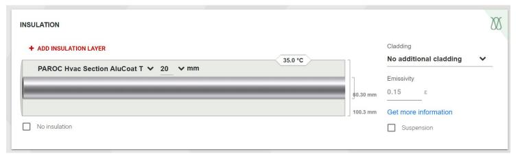
You can add multiple insulation layers. Don't forget to select cladding type, which is very important to determine surface temperature. And support of cladding where applicable.
