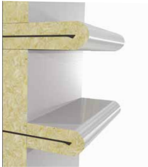
Mat on stiffeners, slabs between stiffeners
