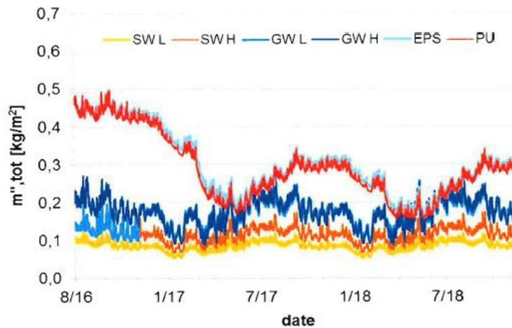
Figure 3. Total mass of moisture in the structure shown during the four months of exposure to the rain and two years after the sheathing. The graph is sourced from [2].
