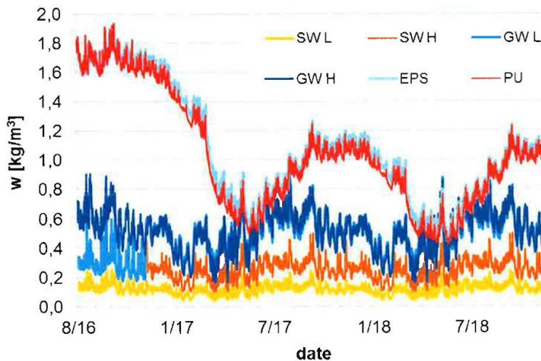
Figure 4. Average moisture content of the insulation material exterior layer (225 mm) shown during the four months of exposing to the rain and two years after the sheathing. The graph is sourced from [2].
