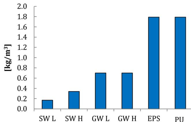
**Figure 2. Initial moisture content at 80 % RH for the thermal insulation materials in the simulations. [2]**
