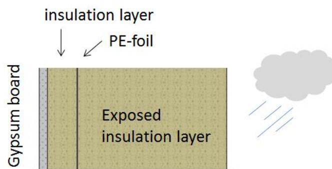
**Figure 1. The unsheltered structure used in simulations using heavy stone wool as an example of a thermal insulation layer.**
