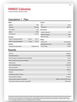
Step 3 Calculation with surface temperature display - cladding systems, suspensions and substructures can optionally be used for the calculation
