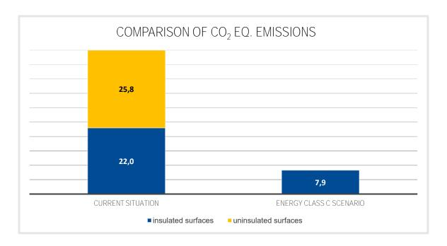
Figure 3: CO<sub>2</sub> eq. emissions reduction if insulation systems are upgraded to VDI 4610 energy class C
