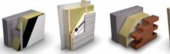
Ventilated facades are characterized by many different system components from different vendors. This can make it difficult for the designer to achieve all the goals set for the structure. In many cases, the design of a façade begins with the choice of façade cladding, after which the structure that supports it is considered, and only finally is the insulation material suitable for the system selected.
