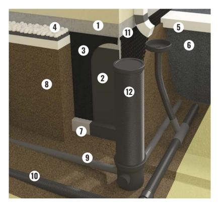
1 Foundation 2 Bitumen felt Foundation waterproofing 3 sheet 4 Ground surface 5 Frost insulation 6 Filling with gravel 7 Geo-textile 8 Sand/gravel 9 Perimeter drain 10 Rain water system 11 **Plastic batten** 12 Drainage inspection chamber
