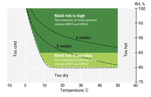
The Finnish Mold Index Model (VTT)
