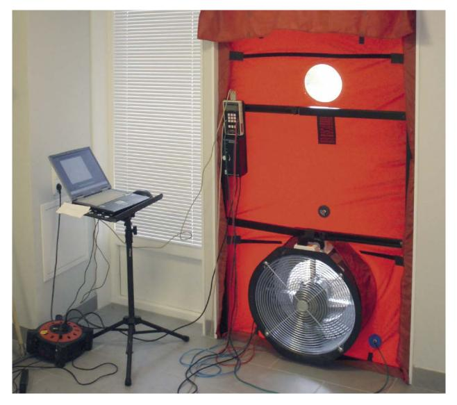
Airtightness measurement detects the building leakage points even before the sealing of structures
