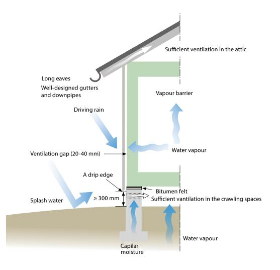
Most of the structural moisture problems in buildings are caused by ground moisture, rain or water used inside the building.
