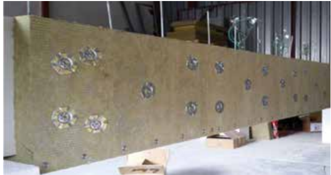
Fire protected concrete beam.
