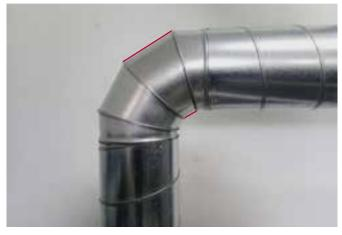
Take the measurements (of the pipeline circumference and the distance on the outside and the inside of the elbow segment);
