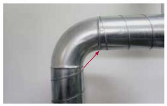
Take the measurement (of the pipeline circumference, chord of the elbow radius measured in the throat);
