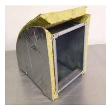
The components of elbow insulation are installed by placing them on the duct surface and matching on the edges while simultaneously piercing the lining with the pins and welding them to the duct surface;
