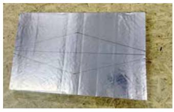
On both edges of the perimeter, on the auxiliary line, mark about 1/5 of the length of the elbow measured at the throat, diagonally, e.g. if the length is 210 mm, the dimension to be applied on both sides should be about 40 mm;
